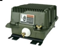
The RF-5382 coupler automatically matches the output of FALCON® II Series HF transceivers to a wide variety of whip, dipole, and long-wire antennas over the frequency range of 1.6 to 30 MHz. The antenna coupler tuning time from memory is less than 150 milliseconds and it operates at power levels up to 150 watts.
